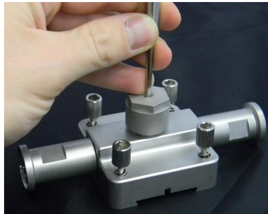
Figure 4-4: Inserting Flow Fibrette into Flow Cell
