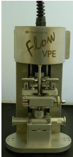
Figure 4-14: FlowVPE with Mounted Flow Cell and Flow Fibrette
