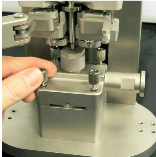
Figure 4-8: Securing Flow Cell to Detector Module
