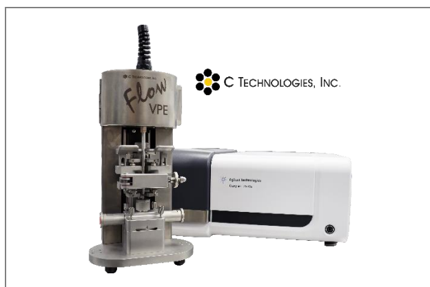
Figure 2-1: FlowVPE and Cary 60 Engine
