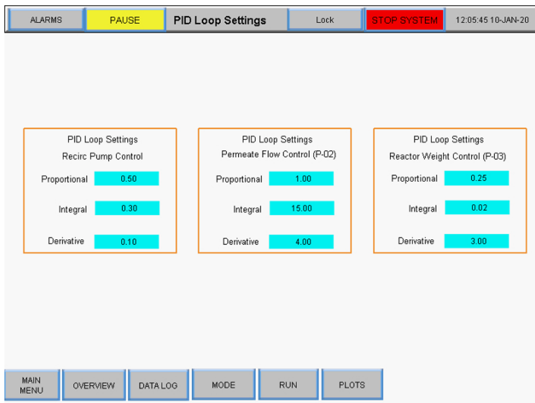
Figure 25. PID loop settings screen
