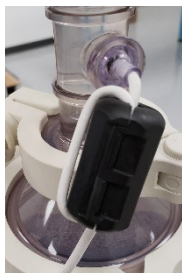
Figure 3. Installed flow path pressure sensor ferrite bead
